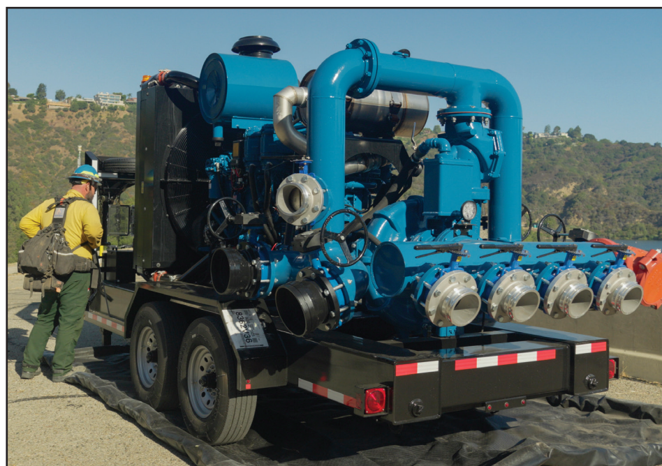
WWS used high-capacity diesel pumps (up to 800 hp each).
